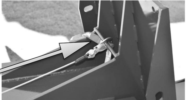
**STEP 5** You may now remove the barriers using the hauler jack or manual tow bar (See *Archer 1200 Deployment Instructions.pdf*). Use the attached winch cable to support movement down the ramp. Remove winch cable when barrier is on a vertical surface.
