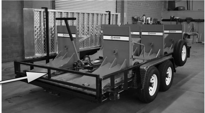
**STEP 2** Two people are required to remove the side ramp. First remove the two wing nuts that secure the ramp to the vertical trailer side fittings. Tilt the highest edge of the ramp forward to lift the ramp out of the lower bracket.
