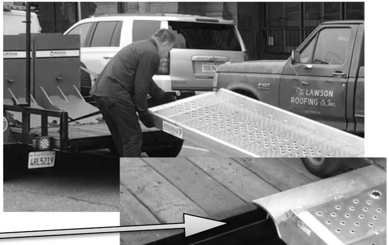
**STEP 4** Before deploying any barrier, first release the winch cable and connect to the winch bar on the top back section of the barrier's vertical plate.
