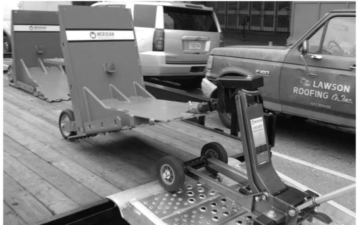
**STEP 6** After barrier deployment, secure all accessories (hauler, tow bar, cables) in the back of the trailer with tie downs. Replace the ramp in the side slot and secure with wing nuts. Replace rear trailer gate rails.
