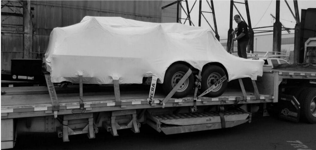
The Trailer Kit containing 8 Archer Barriers, 1 Archer Hauler, 1 Tow Bar, 1 long Arrestor Cable and 7 Short Arrestor Cables will arrive shrink wrapped for its protection on a flatbed semi-trailer. In addition, the trailer is outfitted with a ramp and a winch to assist in the deployment and retrieval of the barriers when they are in the field.
