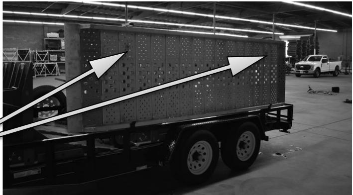
**STEP 3** Place the ramp in the desired location at the rear of the trailer. The top of the ramp has a lip and fitting which rests securely into a channel at the rear of the trailer. The ramp may be slid to the left or the right to align with the off-loading barriers.
